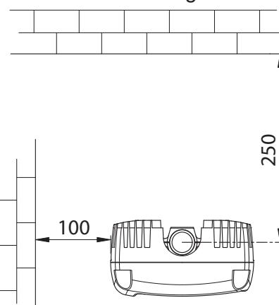
In case of reduced distances connect the frequency converter with the proper unions (see paragraph 16.3.).
